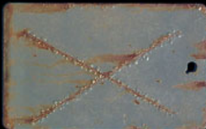
POR-15® System Topcoated with Napa Ruf-Nek HD Spray Paint
