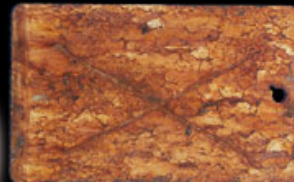
Zinc-Chromate Primer Topcoated with Zynolyte Urethane
