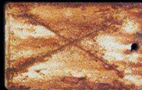
Rust-oleum® Rust Reformer Topcoated with Rust-oleum® Gloss Enamel
